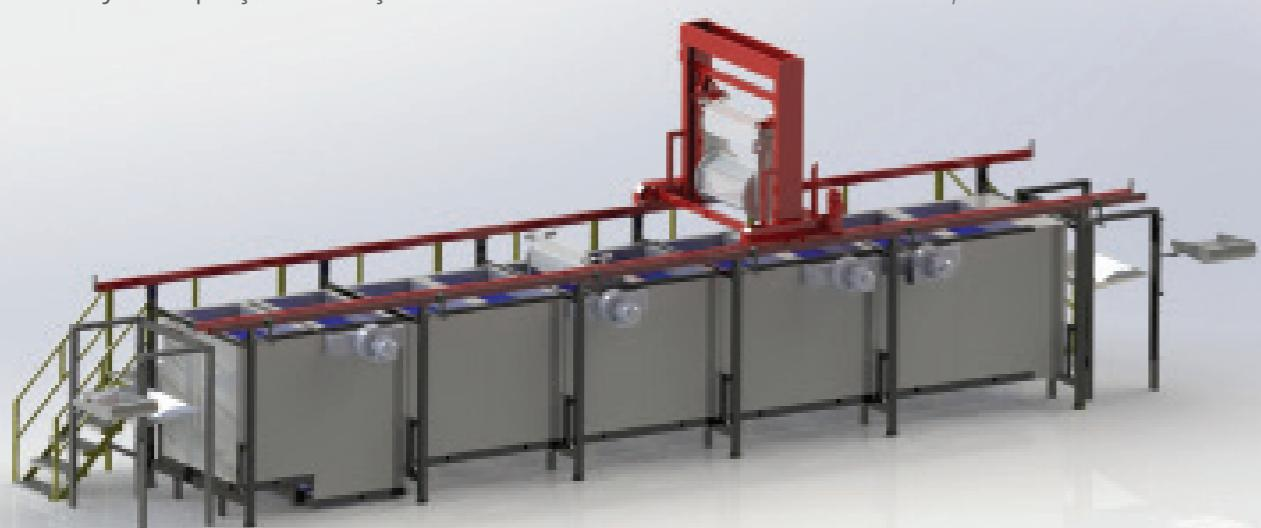
In Dip Tank Lines parts are treated by dipping them inside each process tank for prefixed period of time.
